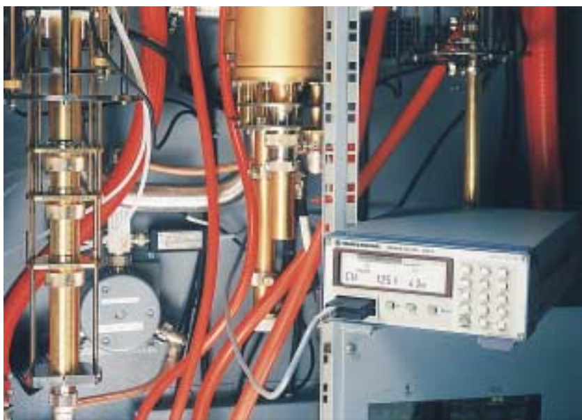
Fig. 1: Power measurement on TV transmitter using Power Meter NRVS
